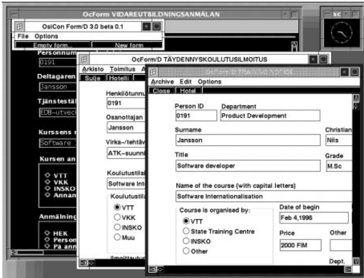
Figure 6. The outlook of OcForm after internationalising it and localising it to English, Swedish, and Finnish locale. In the back, the HP-UX/Motif version is executed with a training notice form in Swedish. In the front, the MS Windows version is executed on the same UNIX machine under WABI Windows emulator, and with both Finnish and English locales.
