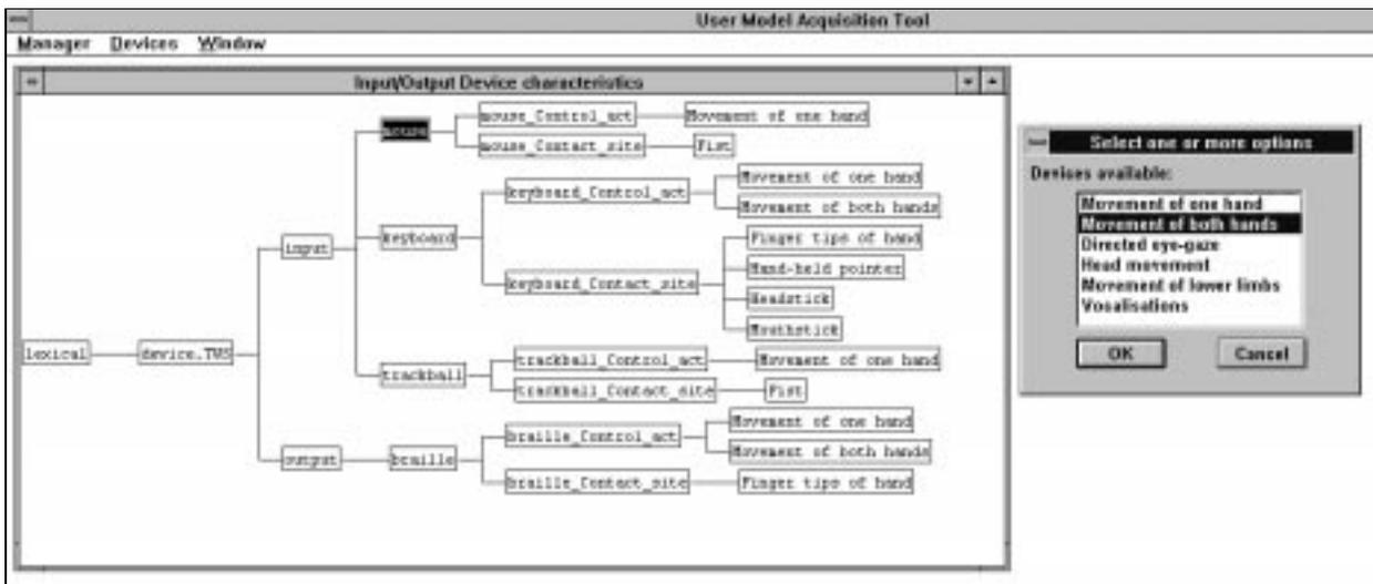
Figure 10: Building device model (Allocating control acts)
